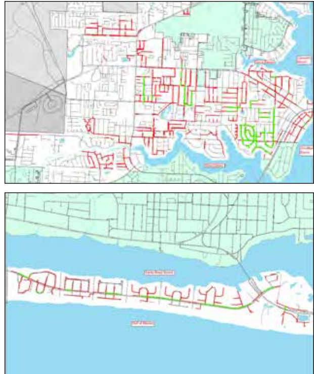
Figure 3-4B. Gravity Mains Proposed for Lining – Ocean City (upper) and Okaloosa Island (lower).
